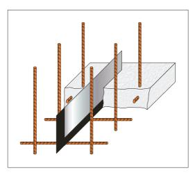
Compared to metal waterstops coated with polymer modified bitumen *FERROTACK* provides some technical advantages. Butyl rubber is a vulcanized synthetic material and has no thermoplastic characteristics such as bitumen. Therefore, *FERROTACK* is much easier to process at very high and low temperatures in contrast to bitumen-coated metal waterstops.
