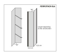
FERROTACK-Stoß and FERROTACK-Eck vertical joint elements are placed on the base plate and bonded to the horizontal FERROTACK joint metal waterstop and fixed each with two fixing clamps type VF. Furthermore the fixing devices of FERROTACK-Stoß and FERROTACK-Eck are fastened with dowels to the precast double wall.
