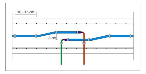
As a rule the air-bleed ends are led out of the construction at a right angle. They may be connected in protective boxes that are fixed to the reinforcement.
