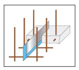
In addition to the *FERROQUELL I* standard there is a *FERROQUELL II* special version available with all-round hydrophilic rubber coating.
